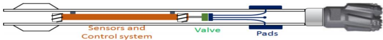
Fully rotating Push-the-bit RSS
